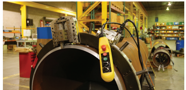
Servo RBL – for RBL clamshells, severs/bevels up to 2" aluminum & alloy piping
