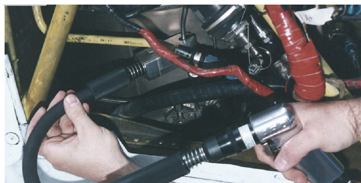
These images show the Model 550's unique ability to perform precision severing of tubes in extremely tight spaces for applications such as aircraft maintenance.
