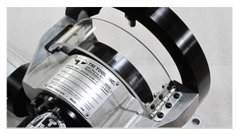
The integral, clear chip guard is designed to provide increased operator safety.
