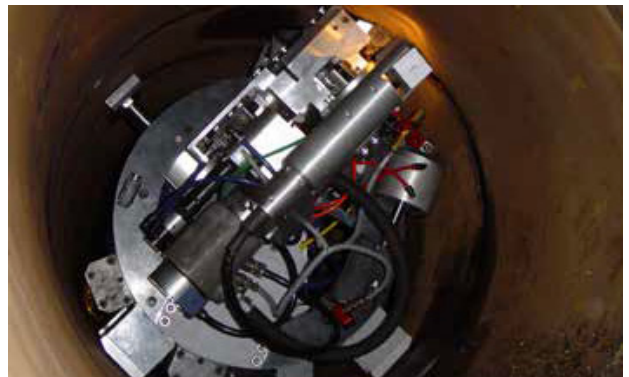
A remote-controlled, self-propelled custom internal pipeline weld profiling system that features laser and video alignment to position and monitor the precise removal of internal weld crowns.
