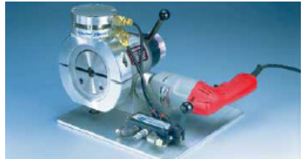
This Model 302 was configured with pneumatic saddle clamping actuation and a quick-detach air fitting for increased cycle times in a high volume tube production role.
