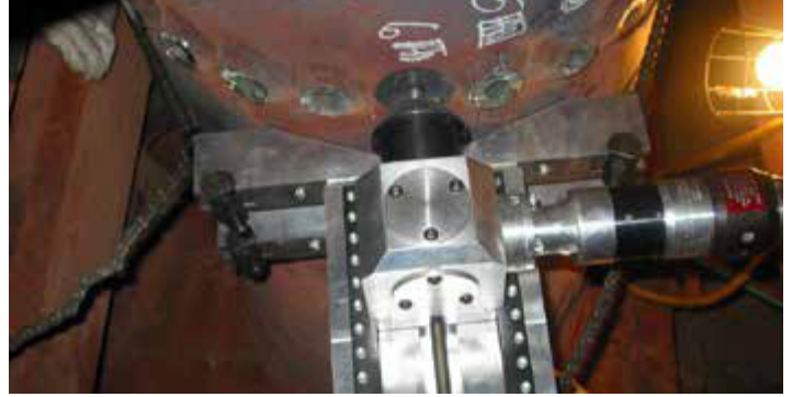
This heavy-duty machine above was designed and built to provide consistent depth and diameter cuts to remove socket welds in a very high-pressure heat exchanger header in a fossil power plant.
