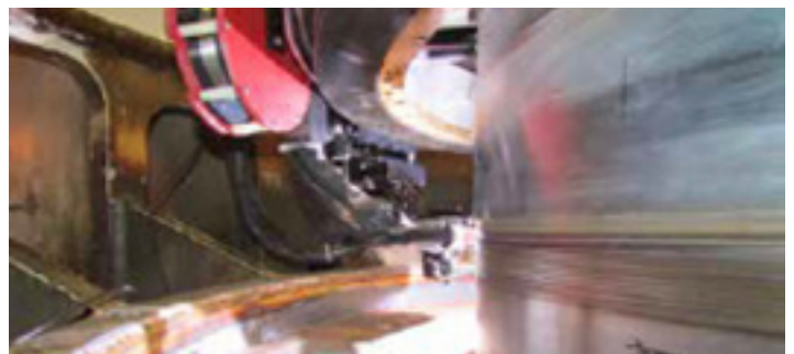
This precision clamshell lathe can be split and reassembled around in-line objects, usually pipe, but in this case a turbine shaft. Our DUALARC® weld head can be seen performing a weld.
