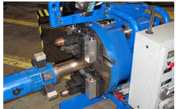
Designed to eliminate weld prep bevel inconsistencies that occur from out-of-round conditions, this pipe facing machine is fitted with custom-built OD tracking tool holders for uniform bevel profiles.
