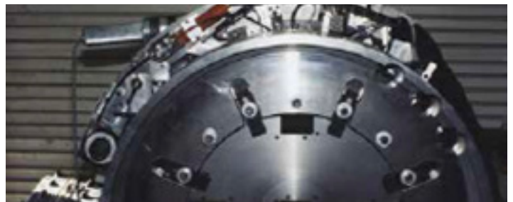
The nuclear industry demands that a wide variety of contingency equipment be kept on site to address any eventuality. This is a custom Omega Seal cutter with video cameras designed for remote operation.
