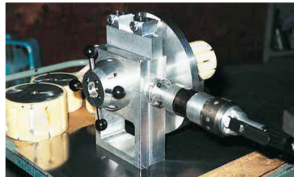
This ID mounted BEVELMASTER® has been custom engineered as a production, bench-mounted end-finishing machine for thin wall tubing with a special base plate and full support mandrel pads.
