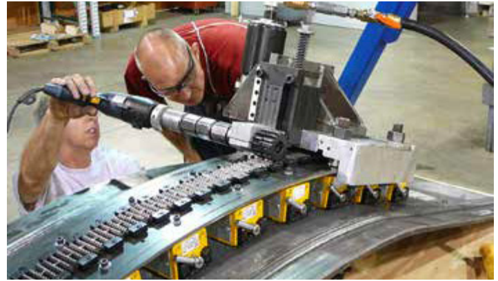
Sometimes it's not just the machine but the mounting system that must be custom manufactured. This special milling machine was designed to be able to conform to the curved side of a ship's hull.
