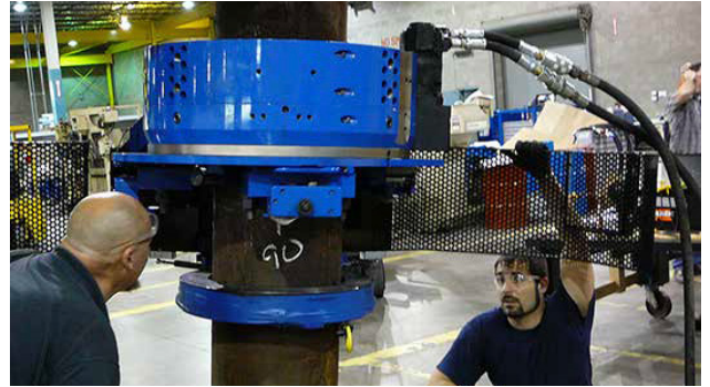
This custom engineered and built automatic-mounting High Speed Severing System was designed to rapidly cut-out defective welds for re-welding in an offshore J-Lay pipeline barge production role.
