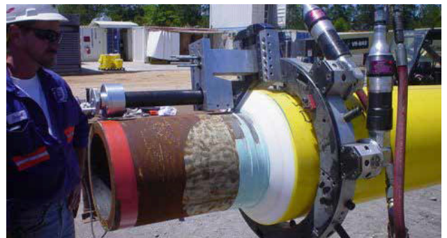
Our fast and versatile RBL split frame lathe was the ideal platform when a customer needed a light and reliable Coating Removal System that featured our custom designed form tooling bits.
