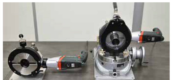
A great comparison shot of the standard (saddle clamping) Model 304, next to a custom 304 with Quick-Lock collet clamping and a special adjustable, offset bed for performing oblique cuts.
