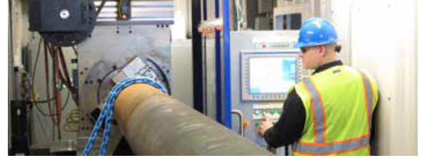
A custom deep counterboring system was needed for a major onshore pipe fabrication project. Our custom system was deployed with a completely custom built pipe rack featuring maximum safety.
