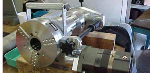
This custom 200 Series BEVELMASTER® ID mounted beveler features a hydraulic drive that is serving dual duty, providing drive power for the cutting head as well as operating an auto-feed system.
