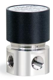
TESCOM BB-3 is a high pressure, low flow, miniature backpressure regulator. Six control pressure ranges are available up to 1200 psig / 83 bar outlet. This regulator can be used for hydraulic or pneumatic service and is small and compact, weighing approximately 4 oz / 0.11 kg in the standard Aluminum construction (316 Stainless Steel also available).
