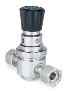
TESCOM 64-3200 Series ultra high purity, high flow tied diaphragm pressure reducing regulator offers  $10\,R_a$  microinch / 0.25 micrometer surface finish and is available in Hastelloy® trim. Maximum flow rates are up to 31.8 SCFM / 900 SLPM, with inlet pressures of 150, 1000, 1500 psig / 10.3, 69.0, 103 bar and outlet pressures up to 200 psig / 13.8 bar.
