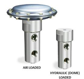
TESCOM 54-2800 Series high pressure, high flow, pressure reducing regulator is designed for hydraulic applications. Inlet and outlet rated up to 5000 psig / 345 bar;  $C_V = 8.0$  for high flows. Air operated and dome loaded versions are available.
