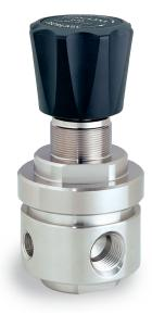
TESCOM 44-3200 Series is a compact, high flow, high purity single-stage regulator for specialty, flammable and industrial gas flows of 5-50 SCFM / 141-1415 SLPM. Diffusion-resistant metal diaphragm seal ensures gas purity and integrity.
