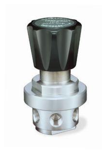
TESCOM 44-2900 Series backpressure regulator is designed to be compact, extremely sensitive and for industrial gases with flows up to 20 SCFM / 566 SLPM. The convoluted Stainless Steel diaphragm provides excellent sensitivity and repeatability; metal-to-metal diaphragm seal minimizes the potential for leakage.
