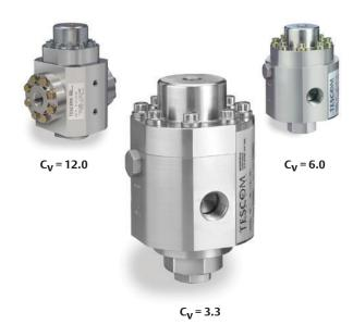
TESCOM 26-1200 Series dome loaded, high flow pressure reducing regulator is externally loaded with 6000 psig / 414 bar maximum inlet and outlet pressures. The 26-1200 Series offers three orifice sizes and  $C_V$  ratings, balanced main valve, and available external sensing.
