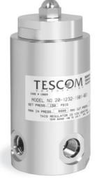
TESCOM 20-1200 Series lightweight, aluminum constructed preset regulator offers an integrated 10 micron filter designed for hydrogen service. NGV 3.1 and TUV batch approved for onboard hydrogen fuel cell vehicles. Excellent choice for other OEM applications.
