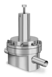
TESCOM 15 Series is designed for ultra high flow applications of up to 28,300 SLPM. The 15 Series is an ultra high purity, 10  $R_a$ , bulk gas pressure reducing regulator. Inlet of 300 psig / 20.7 bar, outlet up to 150 psig / 10.3 bar. Electronically controlled option is available.
