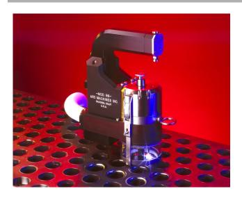
The Model 96 is a compact, automated weld head designed for high-speed, high-production autogenous welding of tubes to tubesheet. Welds made with the Model 96, utilizing the GTAW (TIG) welding process, can pass the most rigid specifications.
