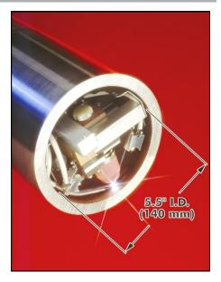
The Model 73 weld head is designed to make butt weld, cladding and weld overlay repairs by remote control on the inside diameters (ID) of piping and specialized valve systems. The Model 73 is a smaller version of the industry standard Model 43 weld head. It is a rugged, field-proven weld head for use in small diameter pipe and other limited radial clearance applications.
