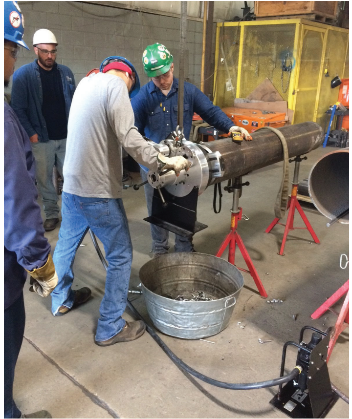
A Tri Tool® BEVELMASTER® ID mounted beveling machine above is performing precision weld prep for equipment training while connected to a PN 75-0115 AIR CADDY™ FRL (Filter - Regulator - Lubricator).
