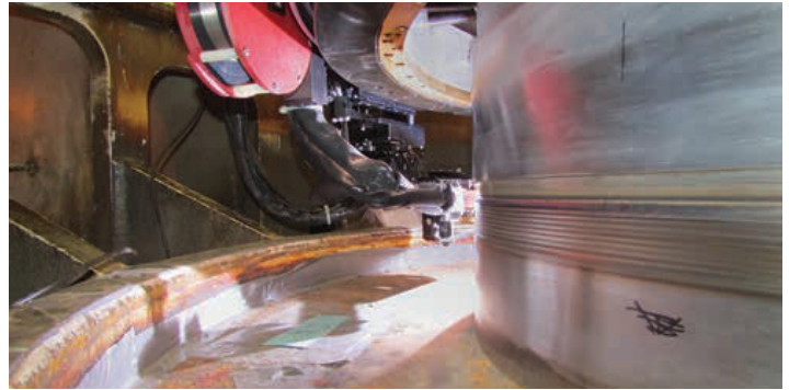
A Tri Tool DualARC® Weld Head is shown mounted to a custom SB Clamshell lathe performing a fill-in weld on a shaft the SB has previously machined.
