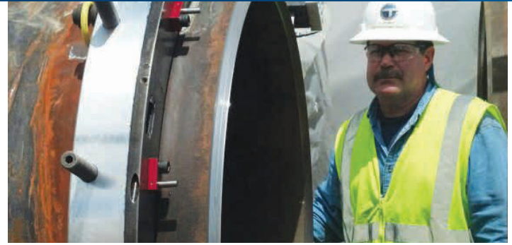
The high performance, second generation RBL-G2 brings improved speed and safety over the field proven RBL series of split frame lathes.
