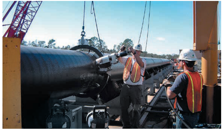
This Clamshell lathe has been configured to perform precision, in-line weld-profiling to strengthen weld joints for offshore platform tendon legs.
