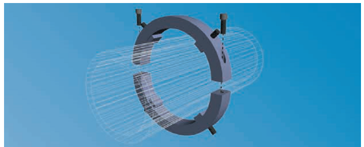
The split-frame design of the Clamshell lathe allows the machine to separate and mount around the OD of in-line pipe or fittings for strong, stable clamping.
