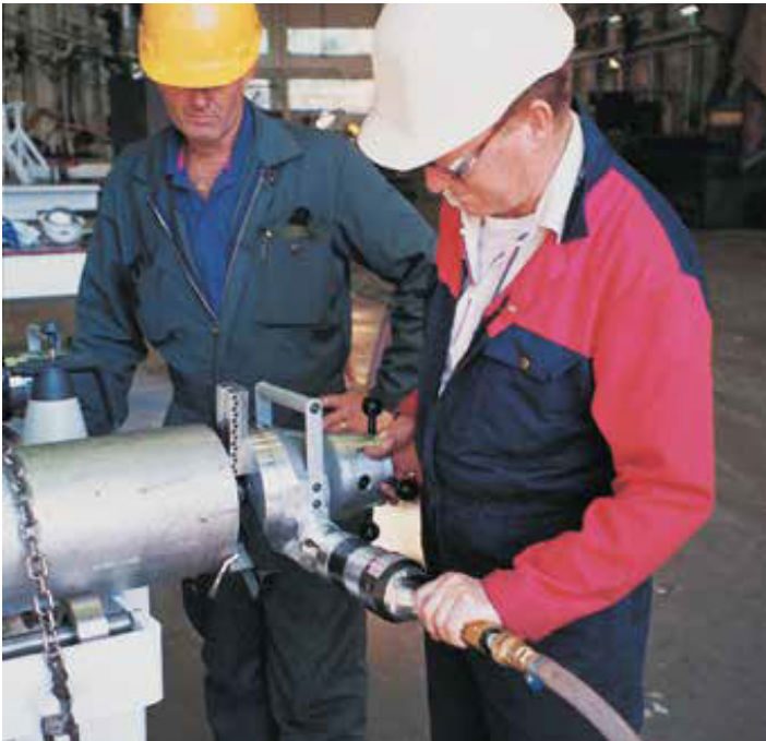
The dependable Model 214B BEVELMASTER being used in a fab shop to generate a precision form tool weld-prep end on stainless steel pipe.
