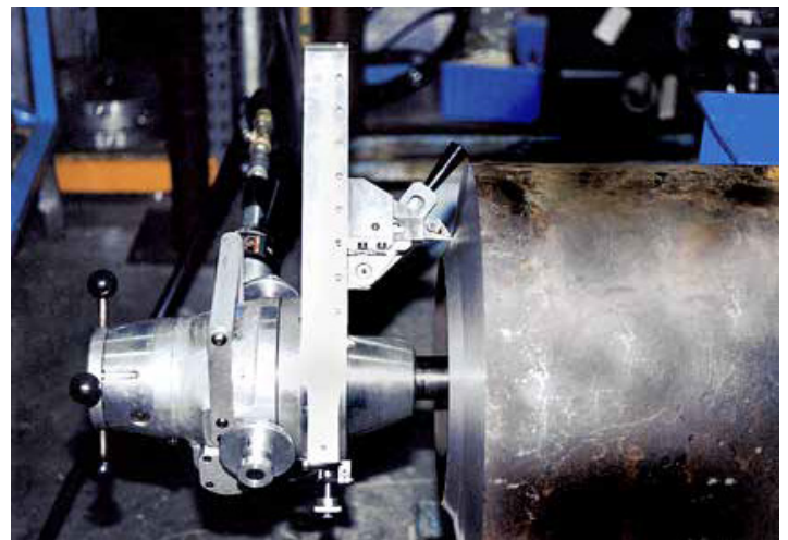
The versatile Model 214B BEVELMASTER with Single Point module generating a precision compound bevel on heavy wall pipe.
