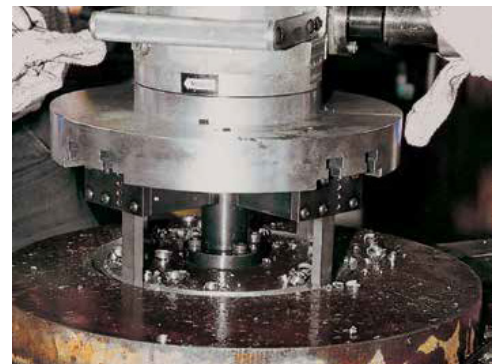
With its power and solid mounting characteristics, a custom BEVELMASTER was perfectly suited for this (four cutting bit) trepanning operation. Note the specially designed bolt-on style mandrel which precisely locates the machine to the work.
