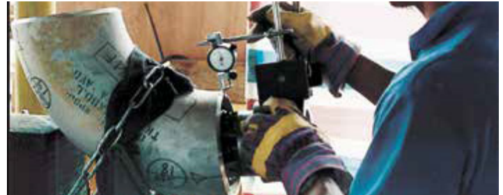
An elbow mandrel head being mounted in a fitting and being aligned with a dial indicator for maximum precision.
