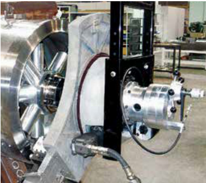
A Model 236B BEVELMASTER has been modified to include an auto-feed mechanism.
