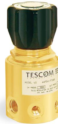
TESCOM 44-1500 Series high flow/low pressure regulator controls outlet pressures up to 600 psig / 41 bar. Large area piston provides accurate pressure control and cycle life superior to diaphragm sensed regulators when applied to heavy duty cycling. Features a segregated/captured vent for hydraulic or pneumatic media and is available in two outlet spring ranges. Optional dome or air loaded versions for remote operation or for use with the TESCOM ER5000 Electropneumatic Controller for automation.
