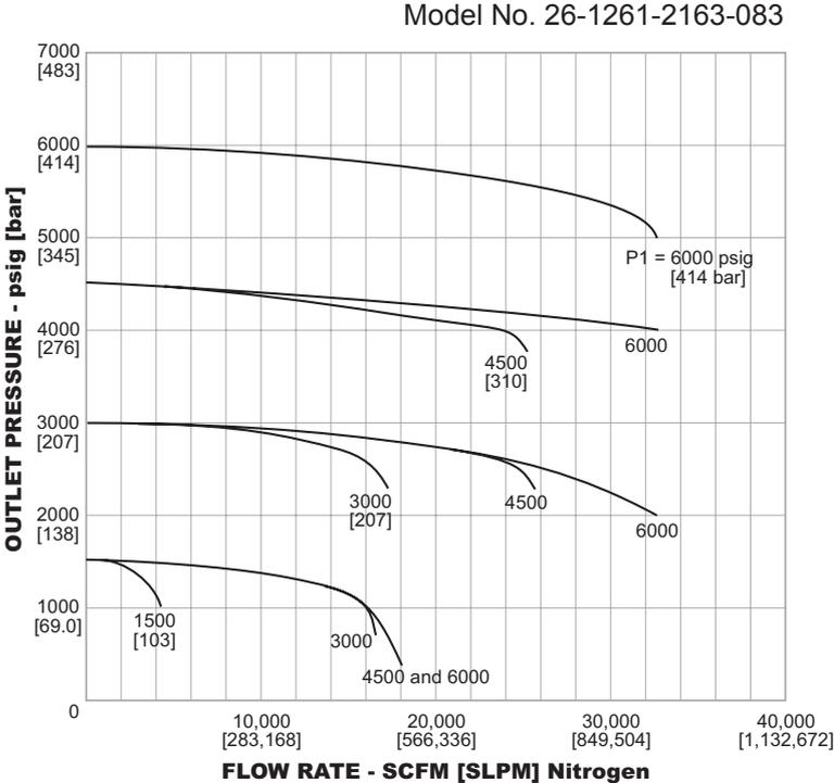
The curves above were generated using analytical methods - error is estimated at ±10%
