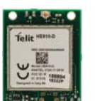
SX1-GSM-001 Cellular Data Modem Worldwide HSPA 3G with 2G GSM fallback
