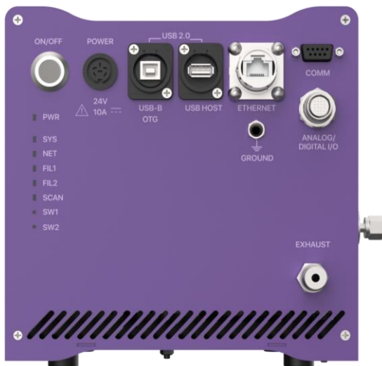
Figure 2. The front panel of AMS. For detailed connector description refer Table 1 and 2
