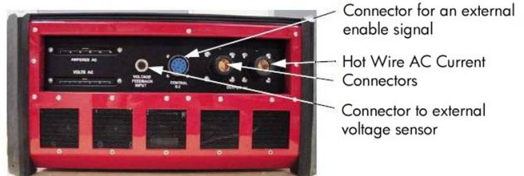
A versatile hot wire welding automation system may be created by equipping an AMI Model 2 weld head with a hot wire torch, AVC, Oscillator, optional Active-Filter Vision System, and the AMI Model 415 WDR Power Supply. This combination can be used for high-quality, high-productivity applications, such as narrow groove welding and cladding.
